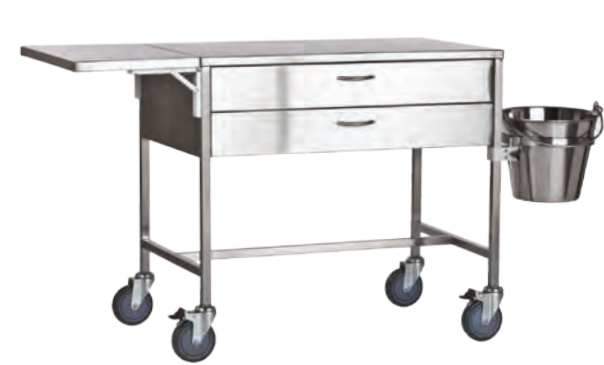
AX 4990 Plaster Trolley 900 x 490 x 900mm Stainless construction 2 Drawers - 125mm deep Drop down shelf / bucket hook
